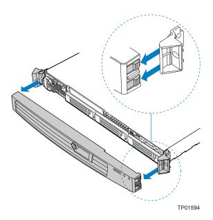
Figure 11. Removing the Front Bezel
